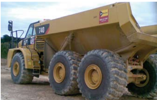
Left side egress of a 40 tonne articulated haul truck.
