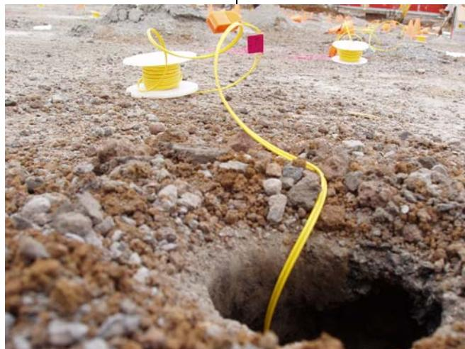
timing, blast design flexibility and improved safety and security. Electronic detonators allow new blasting techniques to continually evolve and Orica's ShotPlus-i™ blasting software assists operators to refine and optimise blast patterns and blast designs, reducing drilling costs and improving fragmentation.
