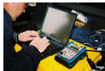
which allows quarry and mining operations to fire i-kon™ blasts remotely. The blast can be initiated from over two kilometres away, enabling personnel to be well away from any safety hazard or other blast effects.
