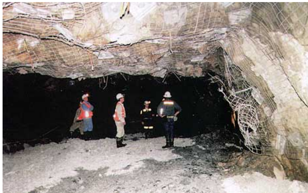
Beaconsfield Gold Mine: A view of the 480 Central stope with backfilling, using a mixture of cement slurry and development waste, in progress. Photo courtesy of Gold Mining Journal.
