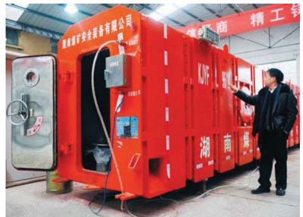
A mining safety chamber to shelter miners during accidents is on display in Changsha, capital of Hunan province, on Monday. It can help 12 people survive disasters underground. Chen Yong / for China Daily
