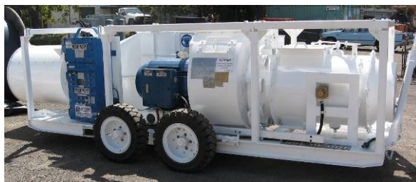
22 cub Auxiliary Fan with a MI Power FLP enclosure
