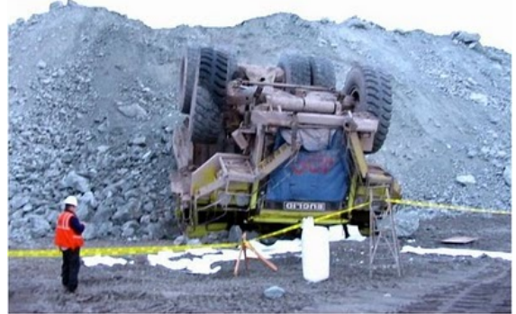
Rear dumper rolled
