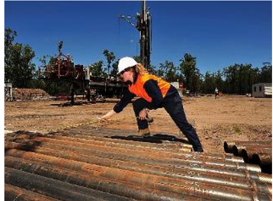
An Arrow Energy employee measures casings used in the drilling rigs at the company's coal-seam gas operations in Dalby, Queensland. Source: Bloomberg
