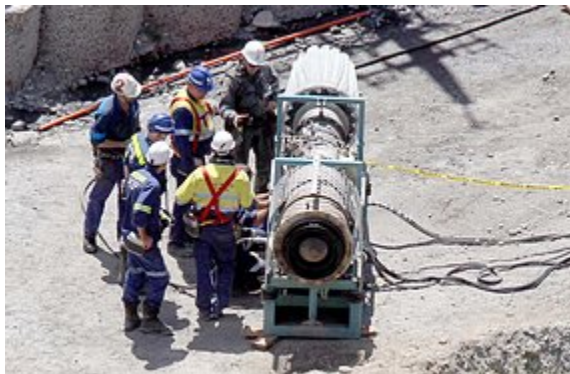
Starting operation: The gag unit is set up at the mouth of the mine shaft (AAP)
