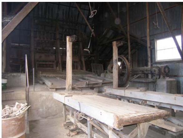
The 10-head stamper battery looms at the back of the shed, with the first set of amalgamation tables leading the residues onto the Wilfley tables in the foreground, all powered by the steam engine on the right. Wentworth Mine, Lucknow, NSW
