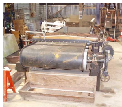
A working Frue vanner at the King Edward Mine Museum, at the former Camborne School of Mines, Truro, UK
