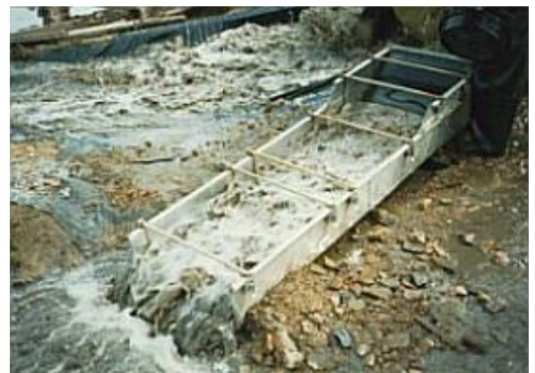
Sluice box in a creek to separate gold from gravels
