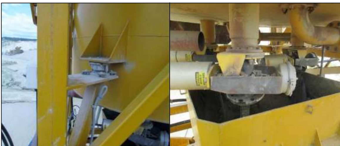
Load Cells measuring the weight of the tub
