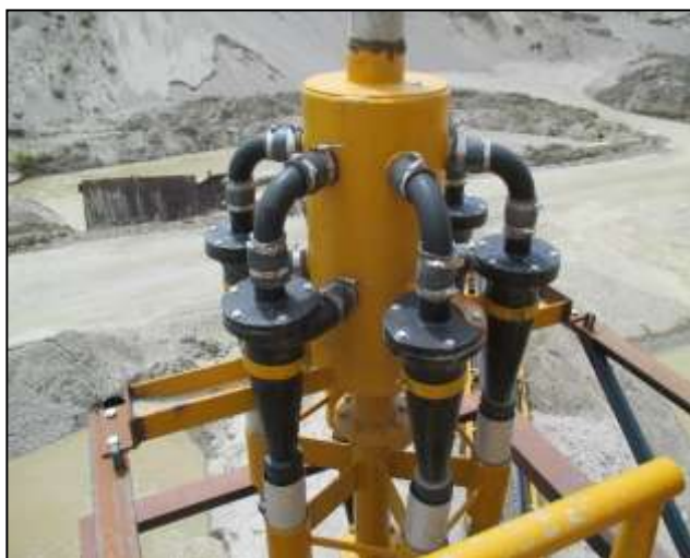
Polyurethane Cyclones to enhance fine sand retention.
