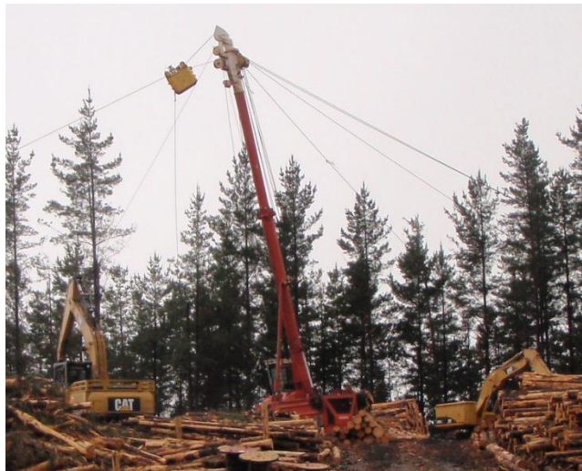
The Madill hauler up top, one Cat machine harvesting and the other stacking
