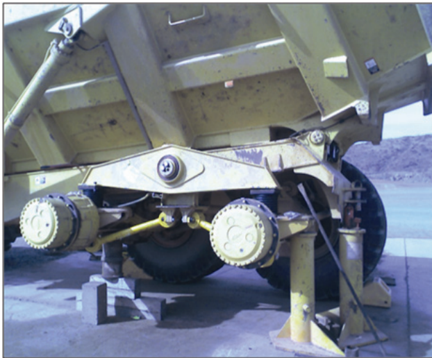
Figure 1 Example of inappropriate use of wooden blocks to support earthmoving equipment
