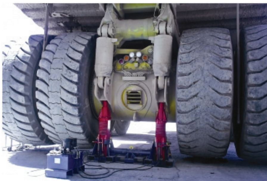
Figure 2 Example of fit-for-purpose jack that can be raised and locked in position to support earthmoving equipment
