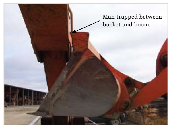
Figure 1 – The bucket positioned as a work platform to clean the boom of the excavator. This is not a safe practice.
