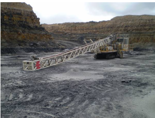
The collapsed drill rig mast (left) and the drill rig's failed pivot point (right) on the RHS tubing.
