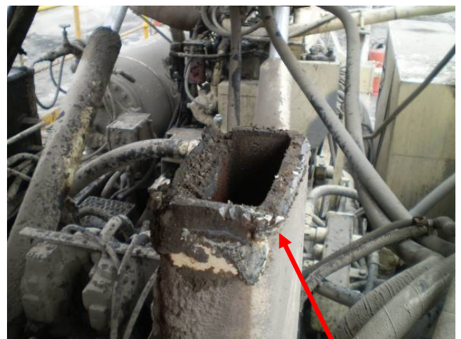
The collapsed drill rig mast (left) and the drill rig's failed pivot point (right) on the RHS tubing.
