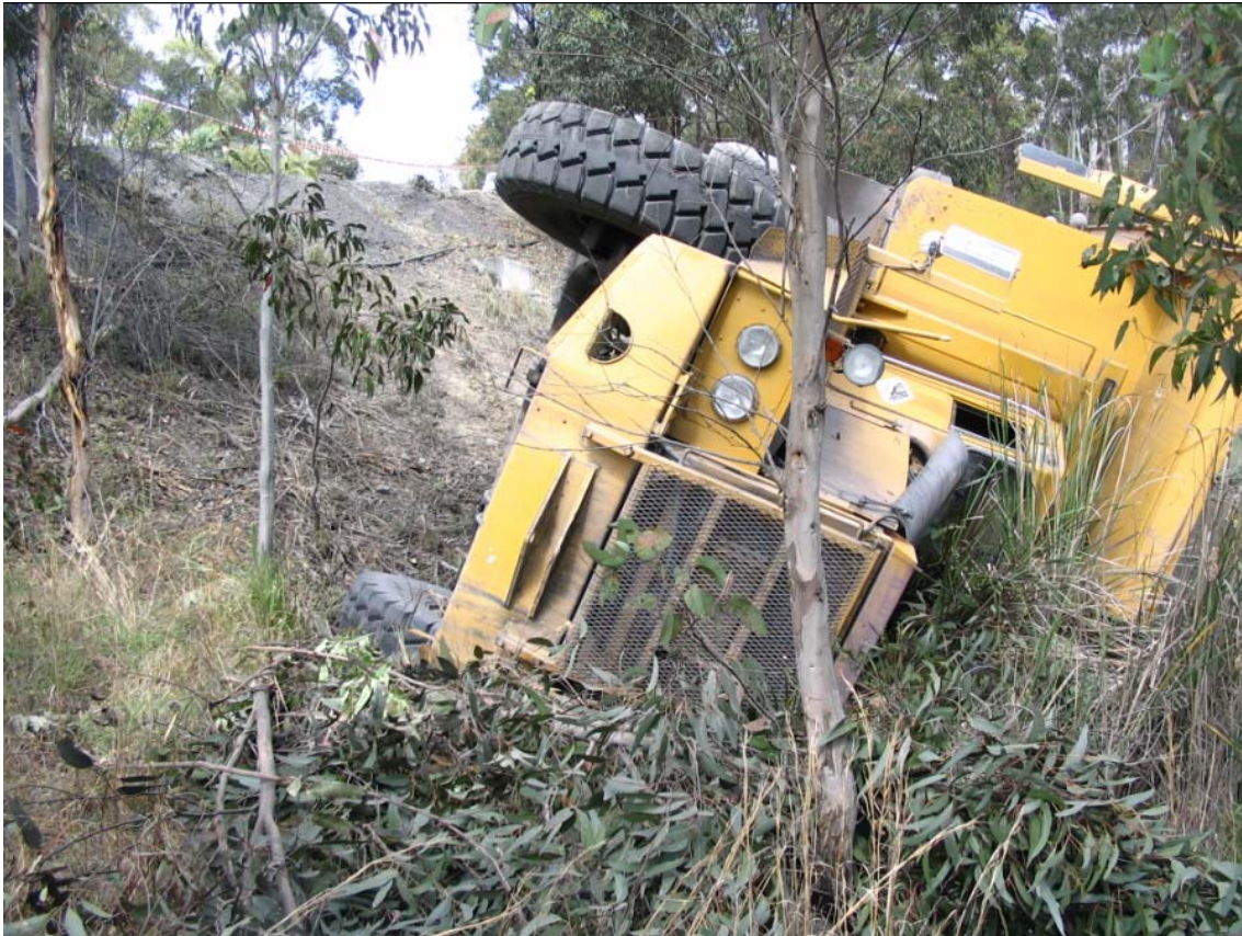
The dump truck lying on its side after rolling over an embankment.
