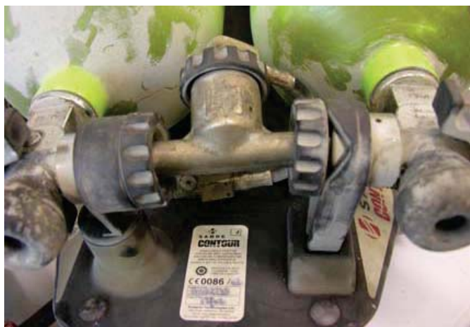
Faulty Sabre CABA unit.
