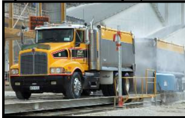
Fig 4. Truck wheel wash using recycled water
